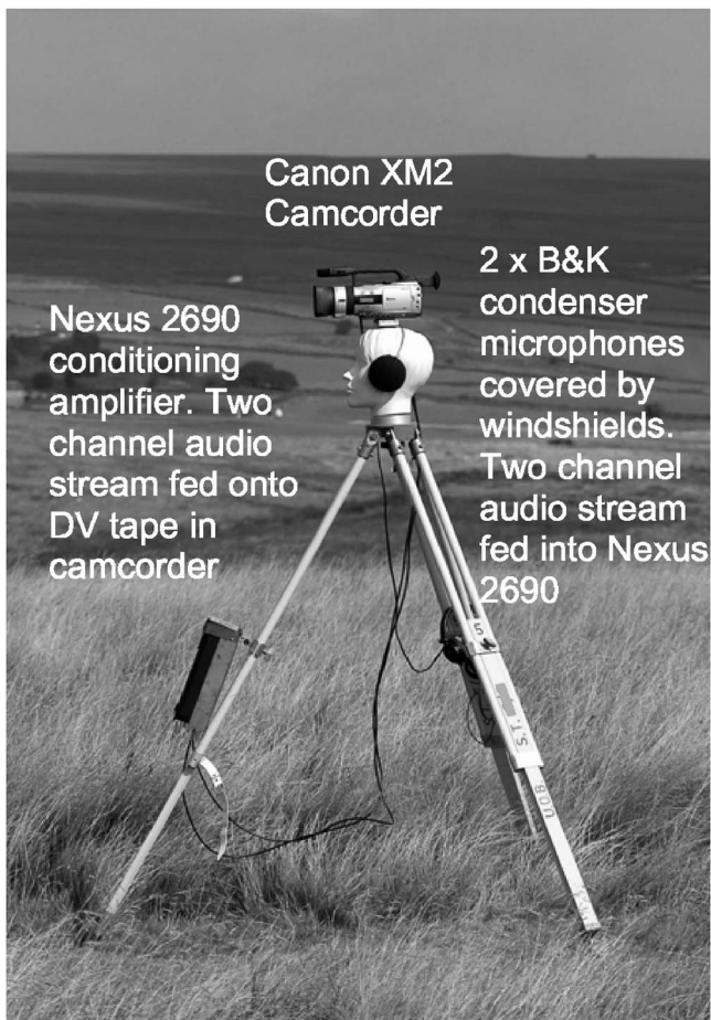
FIG. 2. Recording equipment used to capture the audio-video data.
