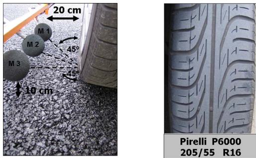
FIG. 1. (Color online) Microphone setup used for the test measurements, showing their positions in relation to the reference tire Pirelli P6000 205/55 R16.
