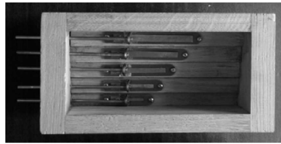
FIG. 8. Physharmonica prototype of Ulrich Aversch (Type I) with five reeds (tone c) in octaves. The scales are similar to the dimensions of reeds for a harmonium with pressure bellows.
